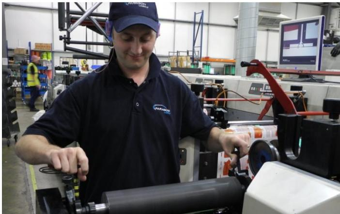
**Operator installing an easy to handle, simple and fast to change Apex GTT anilox roll.**
